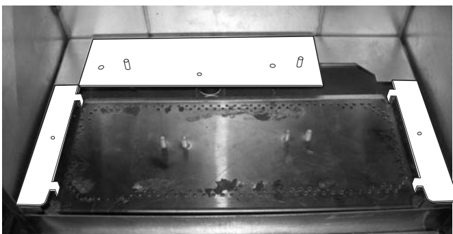
Figure 12. Skirt Extension Plate orientation - Snorkel deflector flange is removed.
